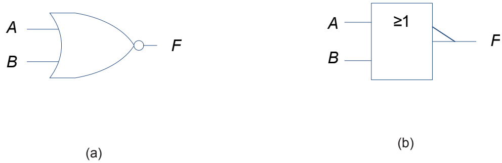
Figure 2.18: NOR gate logic symbols: (a) traditional (b) IEEE/ANSI standard.
