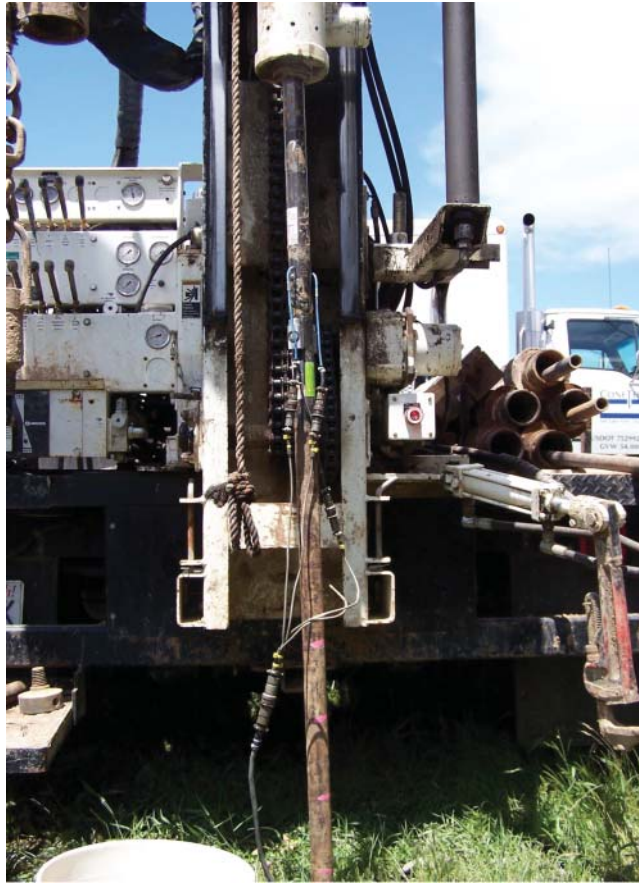
Fig. 2.13 Standard penetration test in progress. (The SPT sampler in the photo is marked to show three 6-inch sections.)
