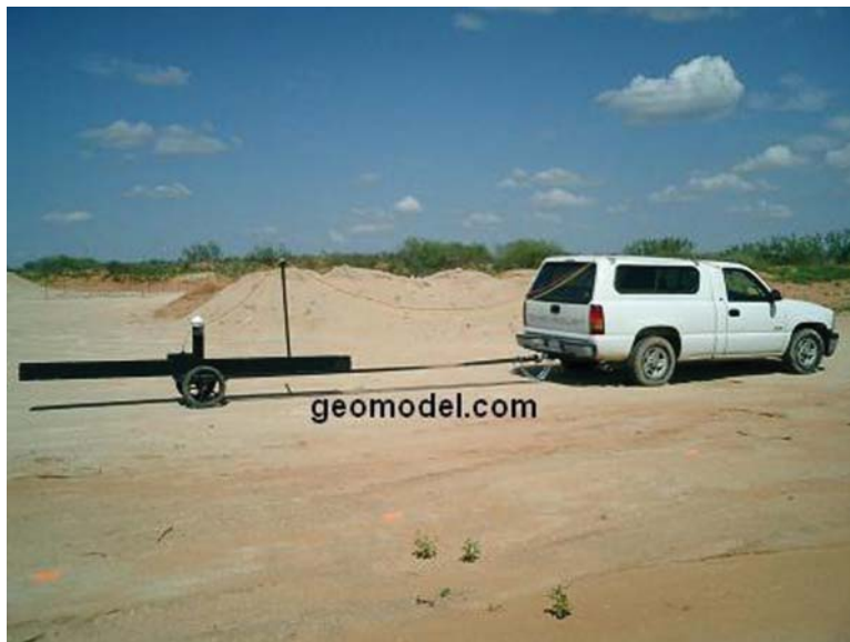
Fig. 2.21 Vehicle-operated GPR truck towing 200 MHz antenna. (Photo courtesy of Paula Turner of GeoModel, Inc.)
