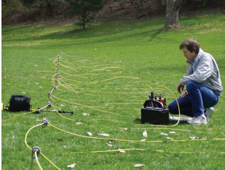
Fig. 2.27 Electrical resistivity imaging survey. (Photo courtesy of Dr. Michael J. Zaleha.)
