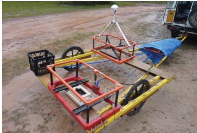
Fig. 2.25 Time-domain electromagnetics survey. (Photo courtesy of GBG Australia.)
