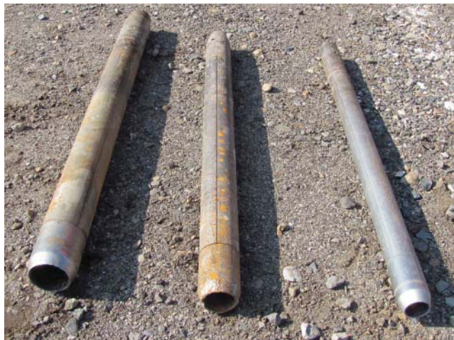
Fig. 2.8 Common split spoon samplers. (From left to right: modified California sampler, California sampler, and SPT sampler.)
