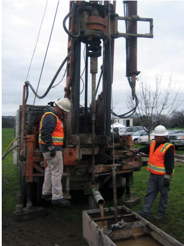
Fig. 2.4 Mud rotary drilling. (Photo courtesy of Martin McIlroy of Taber Consultants, Sacramento, CA, USA.)
