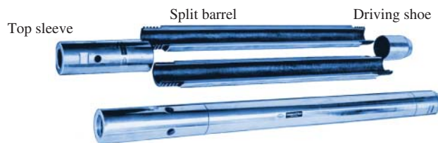
Fig. 2.7 Illustration of a split spoon sampler.
