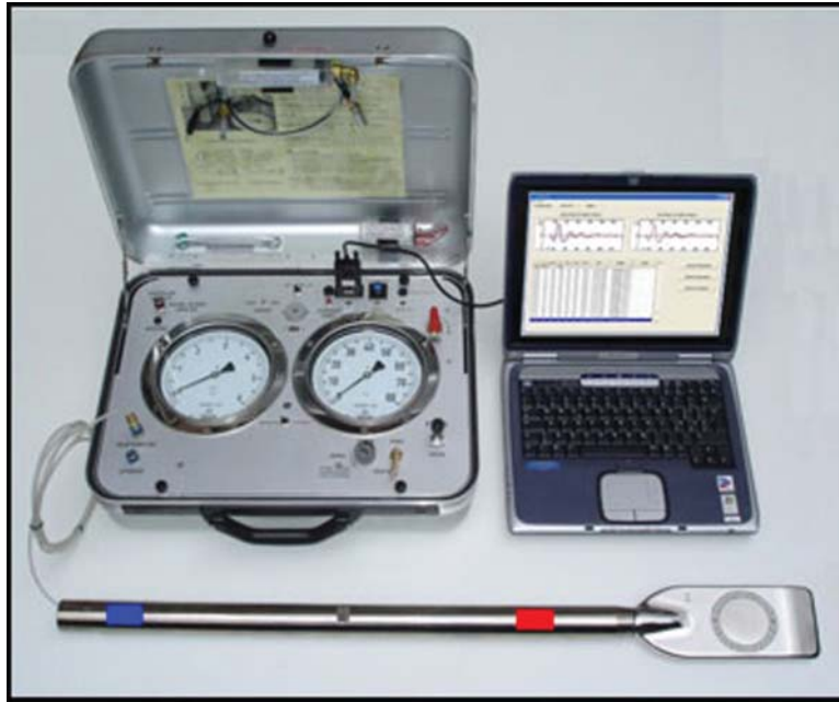
Fig. 2.16 Flat-plate dilatometer test. (Photo courtesy of In-Situ Soil Testing.)
