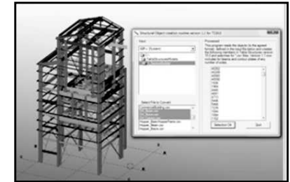
Figure 6.52 Shows an application that has been written to read the values of an Excel sheet which defines the objects – size; grade; orientation; offsets together with its start and end positions. The defined objects are then created in the model as below.
